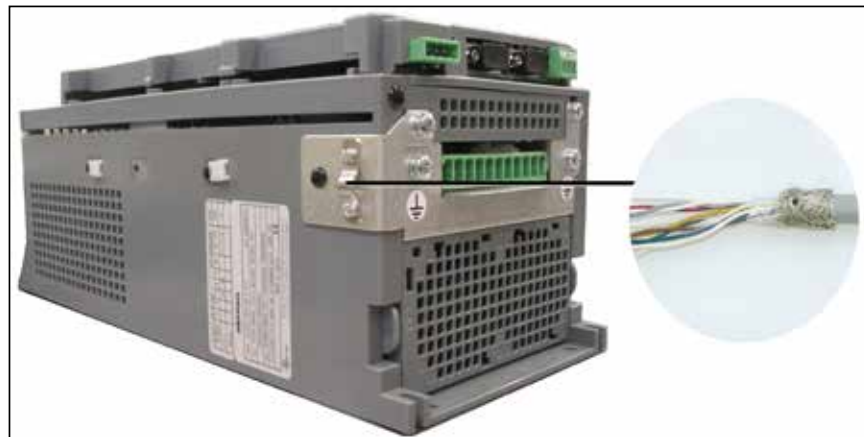
Figure 7.2.4: Connection of shielding (recommended)
